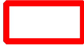
Join Style: Bevel Join
